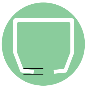
2-degree taper keeps the trolley centered
