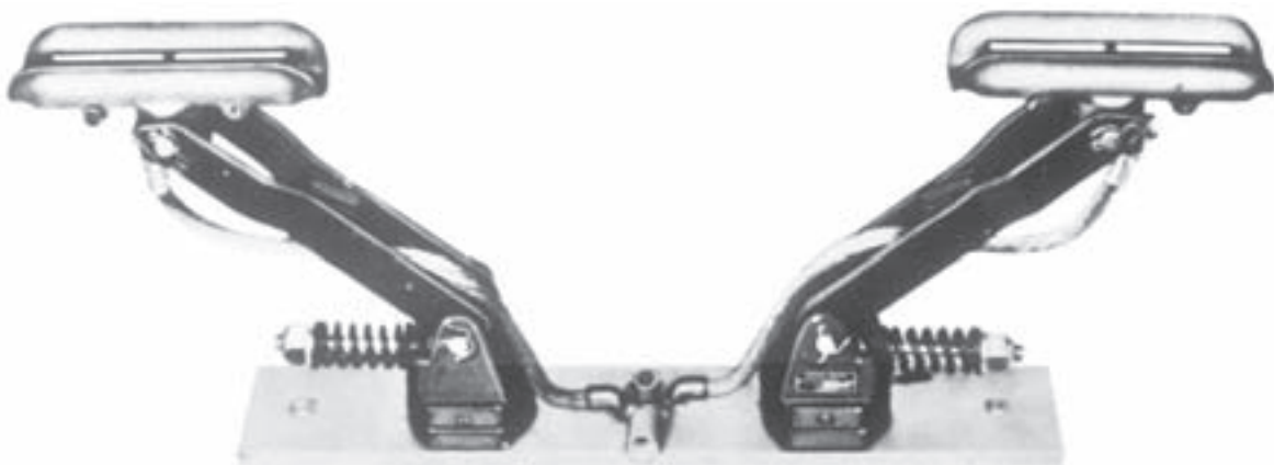
Typical arrangement of collectors in parallel
