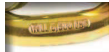
All G70 domestic chain (5/16, 3/8, 1/2) is stamped with the Working Load Limit every 10 links as shown.
