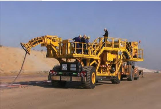
For making cable maintenance- and repair works easier we have developed a cable rewinding trolley for open-cast mining applications. By means of this vehicle the laying, the rewinding onto the large devices as well as the transport of the cables through the open-cast mining area is realized.
