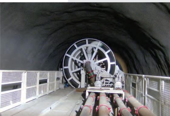
Hose reels enable the supply to mobile pumping stations and spray-irrigation systems for dust reduction as well as the water supply of tunnel boring machines.
