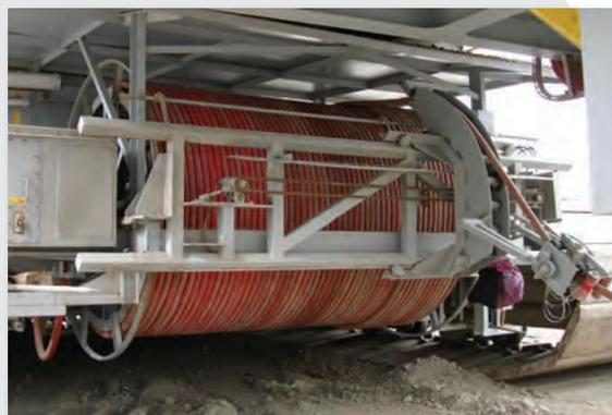
In connection with a spooling device the cable can be reeled on or off the reel body in a controlled way.
