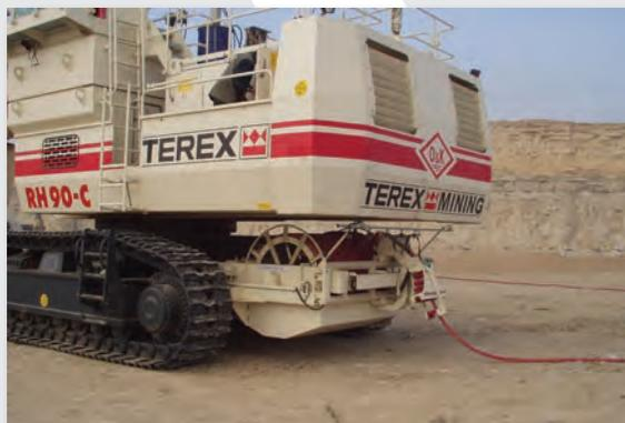
Constantly rising costs for fuel and maintenance of the Diesel-hydraulic drives as well as tightened environmental regulations have caused manufacturers and operators to retrofit their vehicles from Diesel-hydraulic drives to electro-hydraulic drives.
