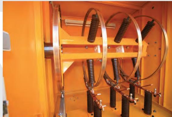
The power- and data transfer from the motor cable reel to the open-cast mining device is effected by our slip ring assemblies. Depending on the case of application these slip ring assemblies are installed in extension of the axle or within the reel body.
