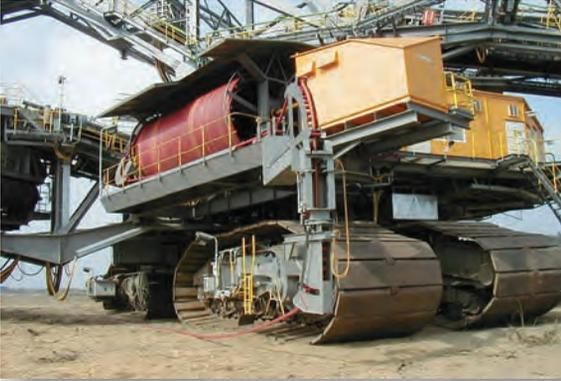
Like for these mobile excavators the energy- and data transfer to the large devices (e.g. open-cast mining excavator or cable storage) also is effected by motor cable reels of *STEMMANN-TECHNIK*.
