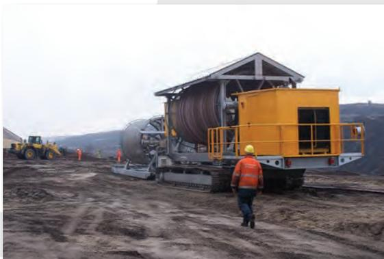
The long distances in the open-cast mining made it necessary to develop special “extension-reels” which if necessary can be placed between the open-cast mining devices and the power supply. The results of this development are “cable storages” and “crawler-mounted cable reels” which allow for the cable storage for open-cast mining devices not having their own motor cable reel and thus increase their operating range.
