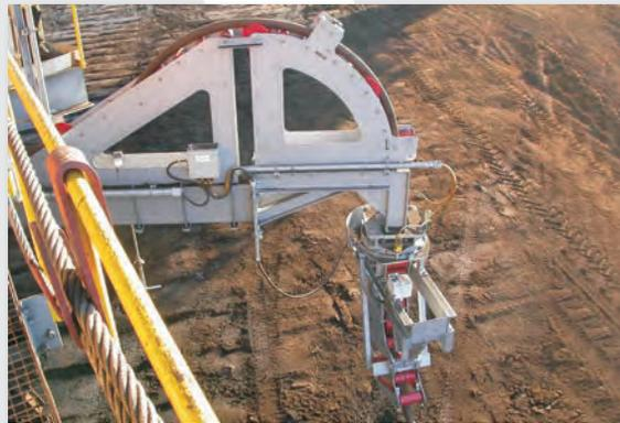
Besides the cable to be reeled the diverting unit is the most used accessory part: It guides the cable into predetermined courses to reel it on or off the reel body in a most cable-sparing way. Frequently, the diverting units are supplied with a tension control. This allows for counteraction in case of a cable tension being too high or too low.
